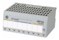
FLEX I/O™ HART modules provide your process automation system with full analog capability and the benefit of HART° (Highway Addressable Remote Transducer) protocol in an I/O module that can be used remotely. The modules offer 8 channels of analog input or output data with accompanying HART digital information.
